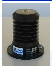
TechImp 12kV Coupler is a capacitive coupler that can be applied for partial discharge measurements. It can be chosen as PD detection sensor for TechImp PDCheck, PDScope or PDBase II systems. It is suitable for on/off line PD tests on rotating machines, for both spot measurements and monitoring applications, in fact it can be permanently installed. A BNC termination is available to connect the coupler through a coaxial cable.
